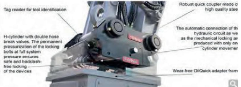
Hydraulic quick change device Oil Quick Original
