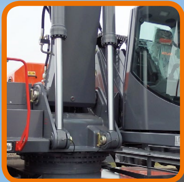
Optimized kinematics for the boom
