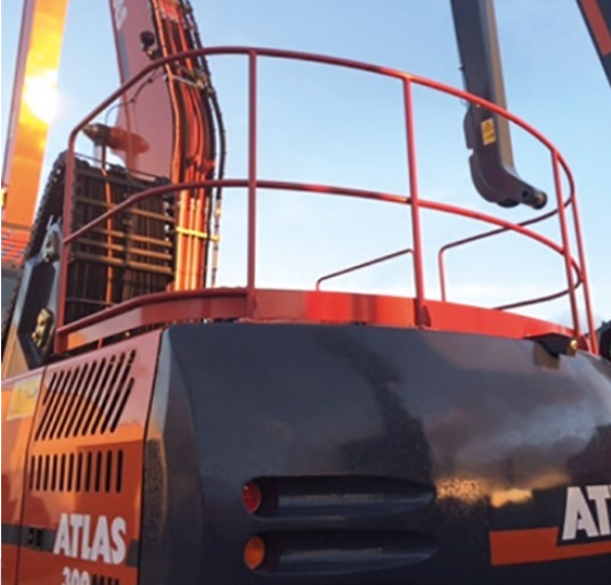
HANDRAIL FOR SUPERSTRUCTURE
