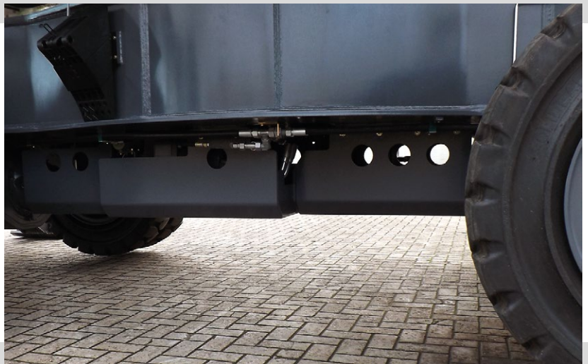
STEEL PLATES FOR THE UPPERCARRIAGE COVER BELOW
