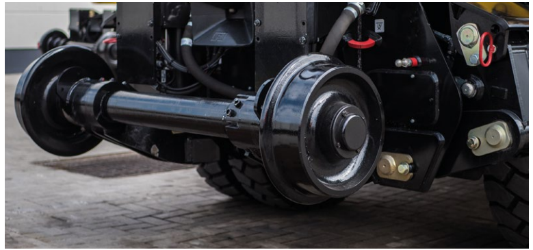
As option available: Friction Drive System available for 1404 ZW-CR with track width 1000 mm.
